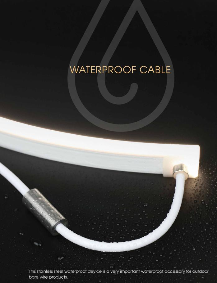
The theory is, by breaking the copper wire, re-welding with interrupter, then sealing the welding joint by mold-injecting high density and high viscosity material, the LED neon strip is completely isolated from the external wiring, realising that the wiring cannot be penetrated with any air or moisture, in spite of the pressure and temperature created by the H<sup>2</sup>O Flex strip.
